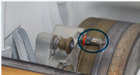
A unique engraving tool, non-invasive for the coating
