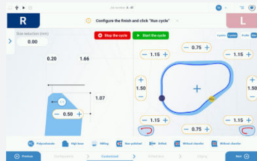
Shape of the bevel (width, height, etc.) defined up to 8 locations
