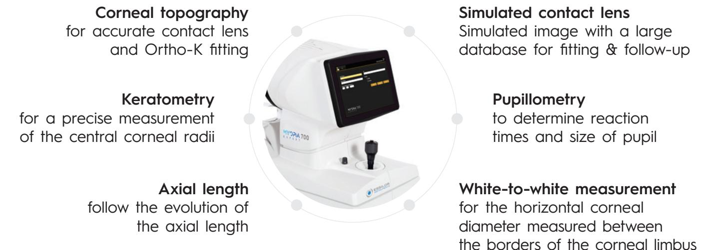
Capture multiple measurements for different myopia control solutions with one single instrument.
