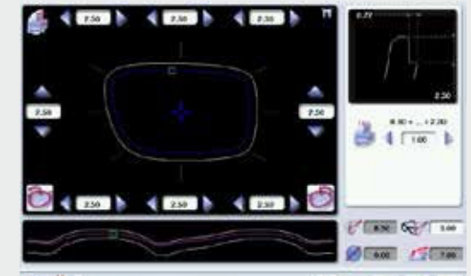
Shape of the bevel (width, height, etc.) defined up to 8 locations
