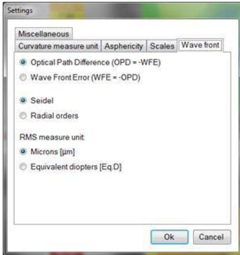
Figure 11-2: Options for the representation of wavefront
