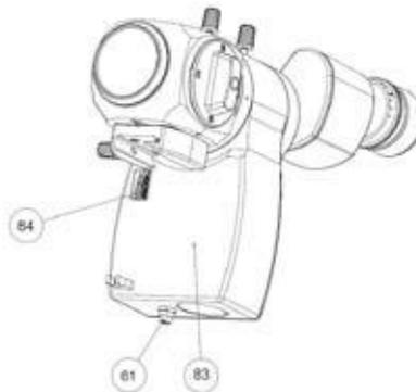
Connect the USB 3.0 cable supplied to the USB 3.0 port (84) on the side of the digital video camera; connect the plug on the other end of the USb 3.0 cable to the USb 3.0 port on computer.
